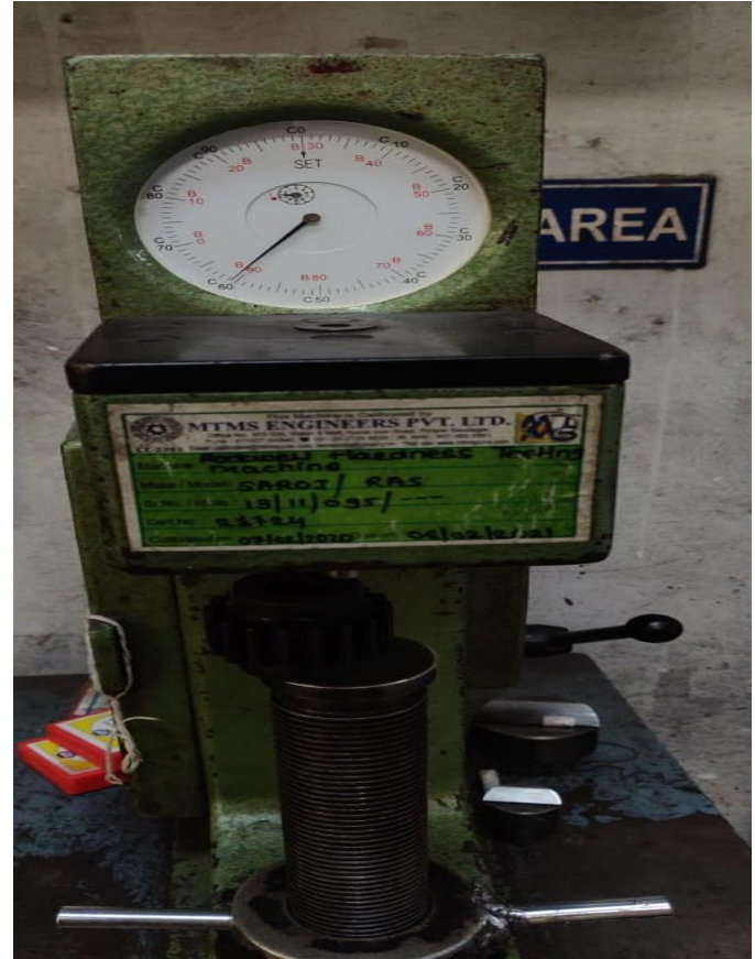
Figure 3: Hardness of 60 HRC of spider gear
