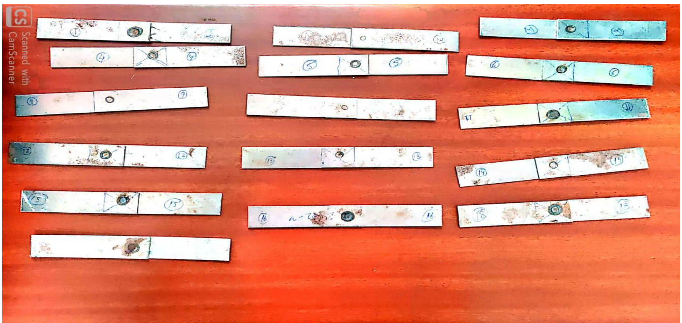
Figure - 2: IF Steel Sheets post Welding
