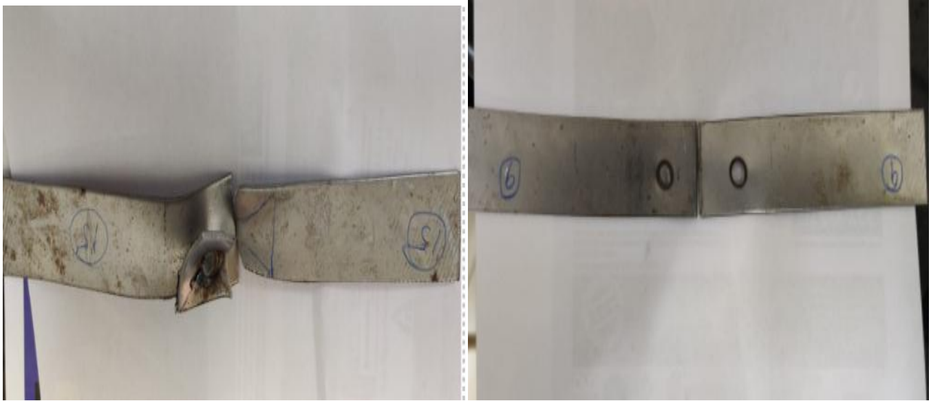
Figure – 4: Weld after Tensile shear strength test
