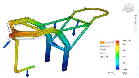
Figure 20 Chassis deformation analysis
