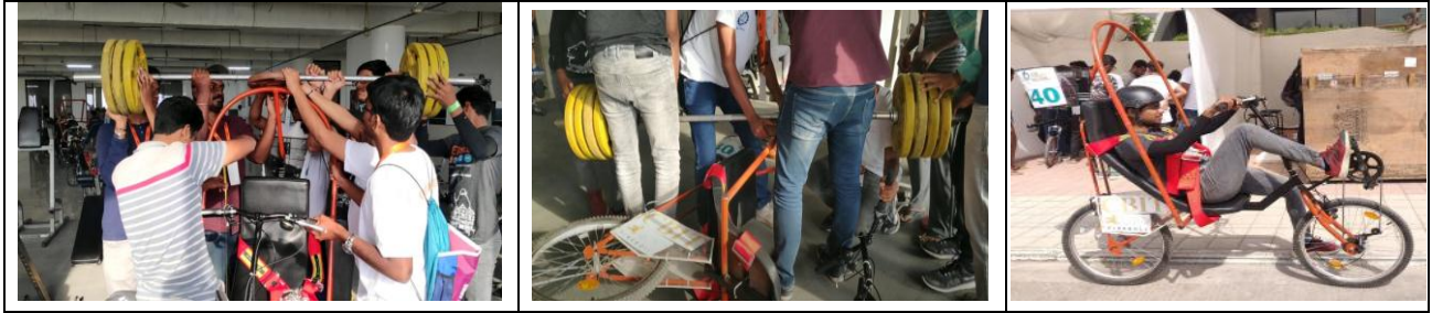
Figure 18: Top load and Side Load Testing
