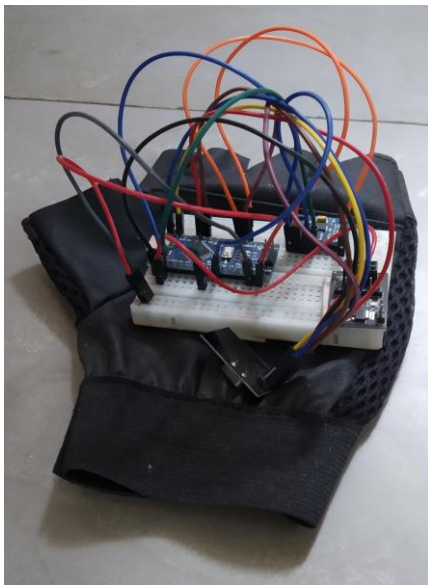
Fig 4: Final Prototype for Hand Gesture Controlled Remote (1)
