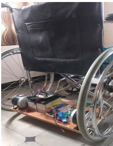
Fig 5: Final Prototype for Hand Gesture Controlled Wheelchair (2)
