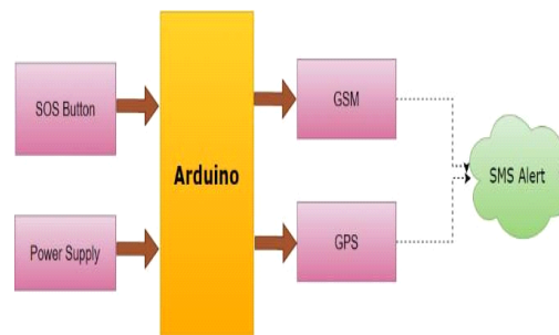
Fig 5: block diagram of GPS and GSM functionality
