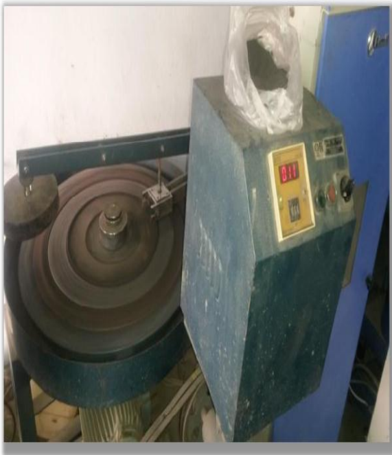
Fig. 6: Abrasion testing of concrete specimen
