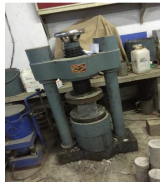
Fig. 3: Specimen being tested on a compression testing machine
