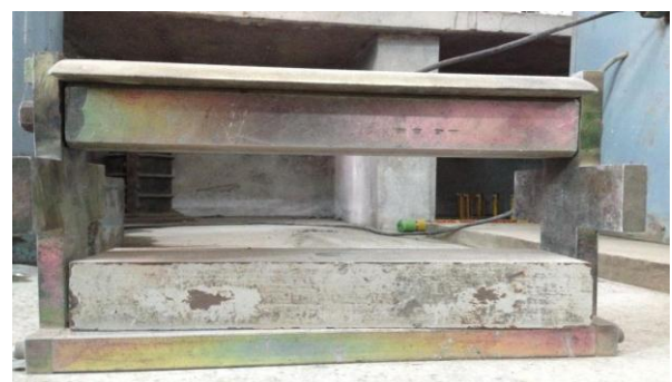
Fig. 4: Gear for split tensile testing of cylindrical specimen
