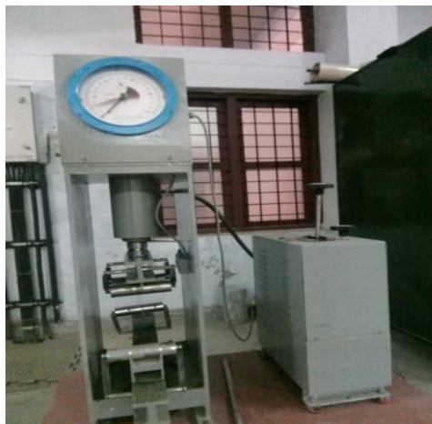
Fig 4.6 Flexural strength test machine setup
