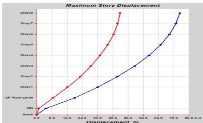
Fig- 7: Storey Displacement of RC Building- LRB and Fixed
