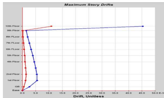
Fig- 7: Storey Displacement of RC Building- LRB and Fixed
