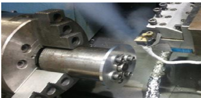
Fig - 2: Experimental set up for cutting operation with cryogenic coolant system
