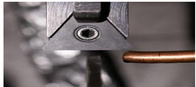
Fig - 3: Nozzle position for cryogenic coolant delivery
