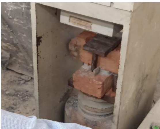
Fig -6: Testing of bricks couplet for bond strength test
