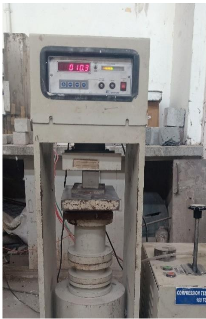
Fig -5: Compressive strength of mortar
