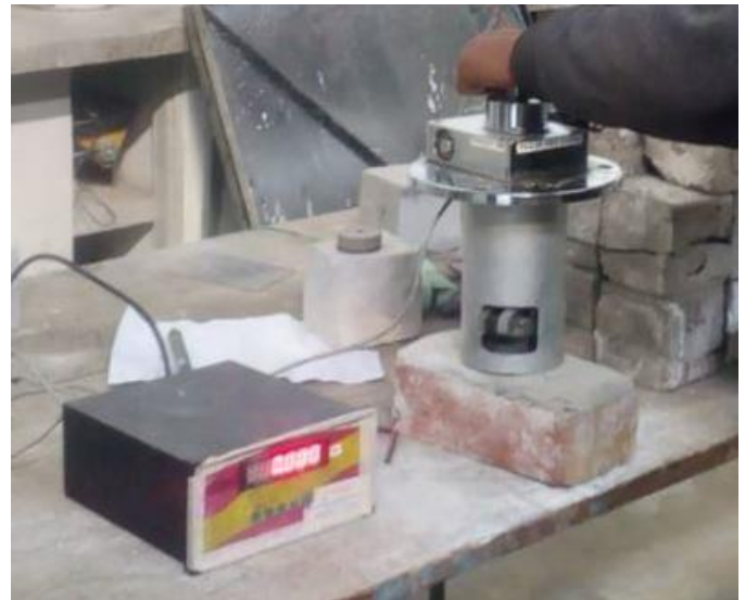
Fig -7: Testing of adhesive strength of cement mortar
