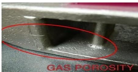
**Solution:** Check whether dies are clean and sure a metal alloy are dry and ingot. A sufficient sprue and runner length will help molten metal to flow stable and discharge the gases. Used high quality mold releasing agents and reasonable amount is to be used.
