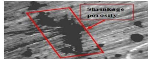
**Solution:** Adjust the temperature of casting to reduce total volume deficits. Redesigned of gate or runner system to have riser that are enabled to flow molten metal continues. Improve casting structure overall. Increase heat dissipation for ribs, cooling coil and insert internal chills.
