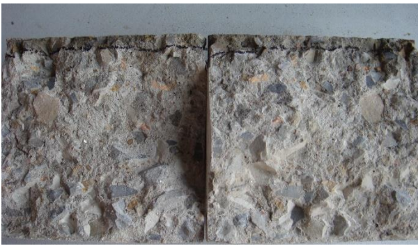
Figure 13 - A typical shape of split cylinder
