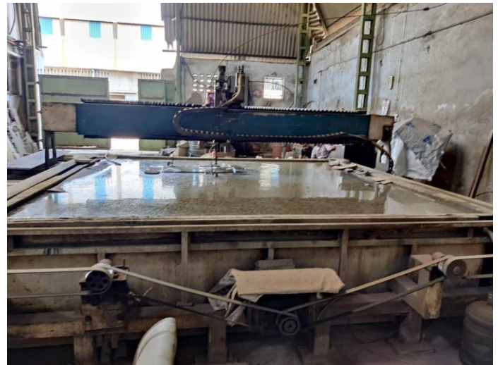
Figure-1: Experiential setup of AWJM process used in current study
