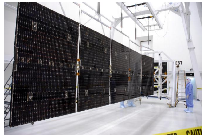
Fig -7: Multi-junction panel of Dawn spacecraft
