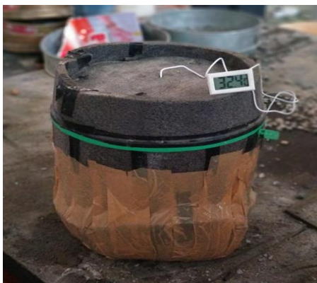
Experimental setup for measuring thermal conductivity of mortar cubes
