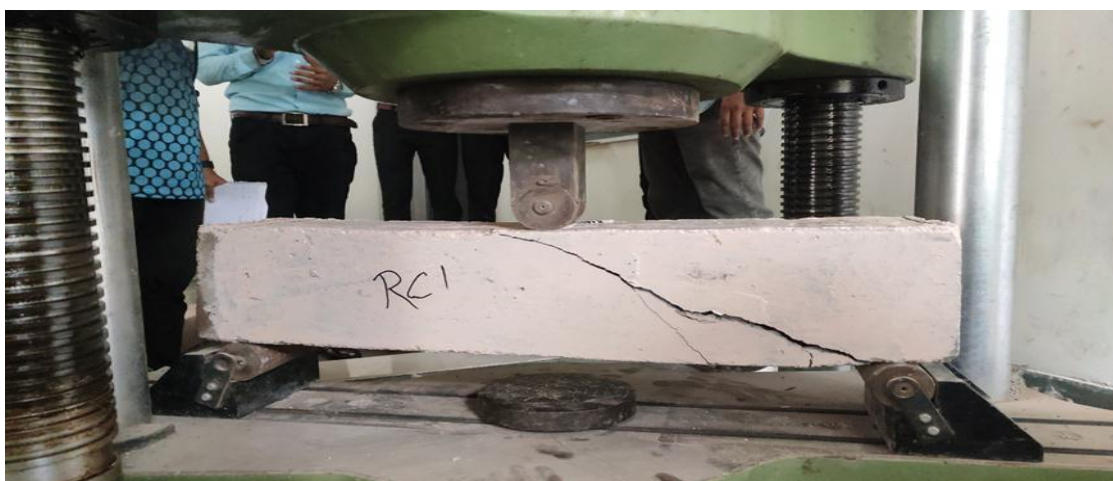
Fig -1: Overview of the ultimate test setup in UTM.
