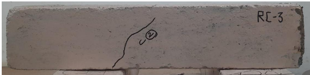
Fig -9: Cracks developed on longitudinal section of RC- 3
