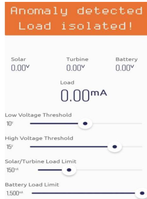
Fig-17 : An alert message for undervoltage condition
