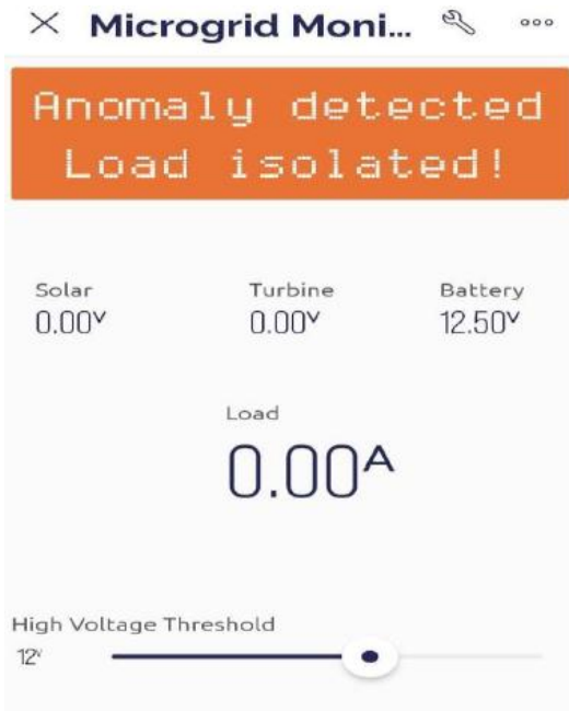
Fig-16 : Display in Blynk server during overvoltage condition
