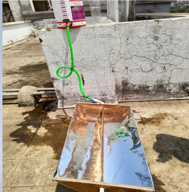
Fig -3: Solar Parabolic Trough water heater
