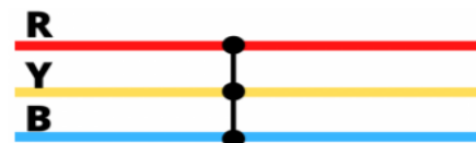
Fig-2: Three Phase Line to Line Fault
