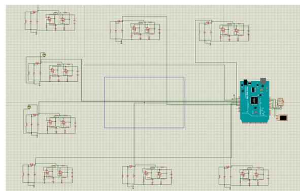
Now we have connected all 8 Chua's circuits in parallel to generate an 8-bit random binary signal.
