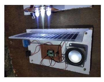
The receiver side consists of Photo detector, amplifier and a speaker. The digital data is received by the photo detector and it converts digital data into the electrical signals. The electrical signals are then passed to the amplifier circuit to strengthen the signal if in case if there is attenuation of the signal. Finally, the audio is played at the receiver side by the speaker.
