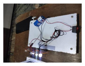
The transmitter side consists of a power supply, audio jack and LED.
