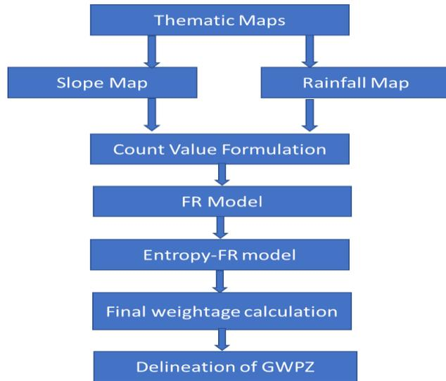
**Fig.1** Flow chart for Methodology to be followed to Identify Groundwater Potential Zones
