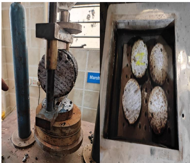
Fig 3: Mould kept for testing Fig 4: Moulds kept under water bath
