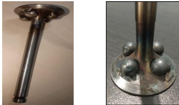
Figure -3. Modified Inlet poppet valve (4 Ball valve)
