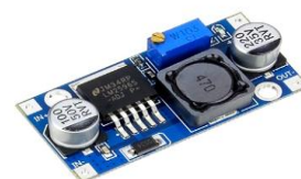
Fig 6: DC-DC Buck Converter.
