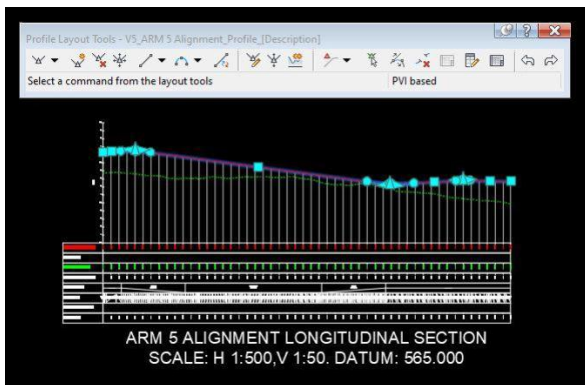
Fig -10: Creating a Vertical Profile using Profile Creation Tool.
