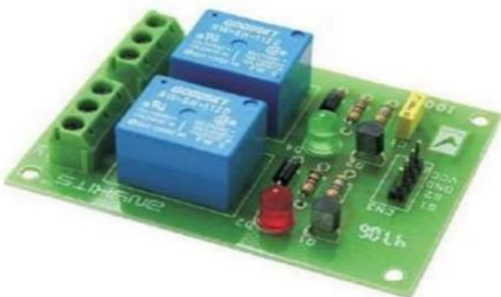
Figure 7: Relay Motor Driver
