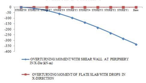
The restraining moment for building with shear wall at periphery is more as compared to building for flat slab with drops. According to IS 456:20000, Cl. 20.1, structure stability in the event of resisting moment must be larger than 6/5 times the maximum moment due to the normal dead load and greater than 7/5 times the typical applied loads.
