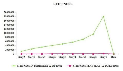
The stiffness of model with shear wall at Flat slab shows lower stability as compared to model with at periphery. Thus At periphery provides more stability to building under lateral loads.
