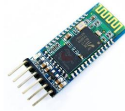
Fig 7: HC-05 Bluetooth module
