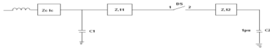
Fig 1. Equivalent circuit of GIS
