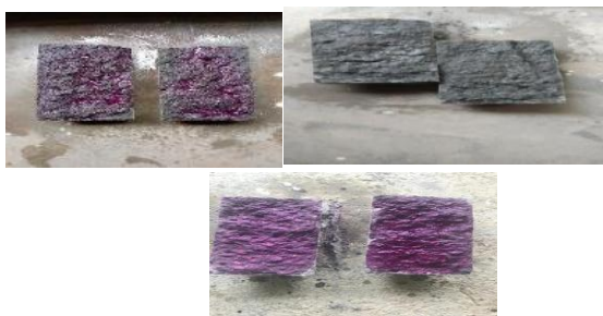
Fig -4: Carbonation Test
