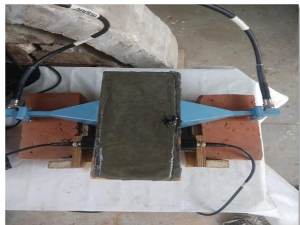
Fig -4: Experimental Setup Sketch for Testing Fresh Concrete
