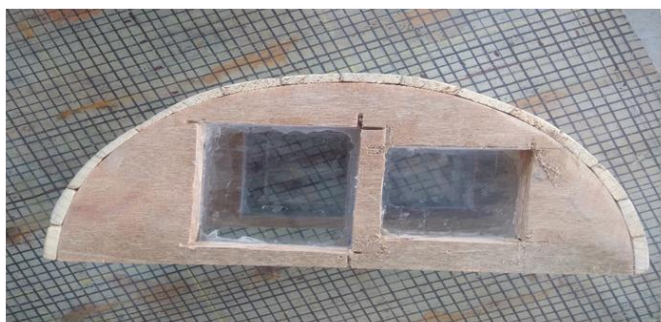
Fig -2: Mould for Fresh Concrete Testing.
