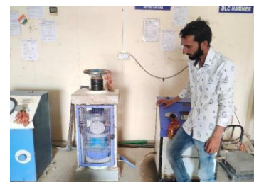
Fig.12-Split Tensile Strength Test
