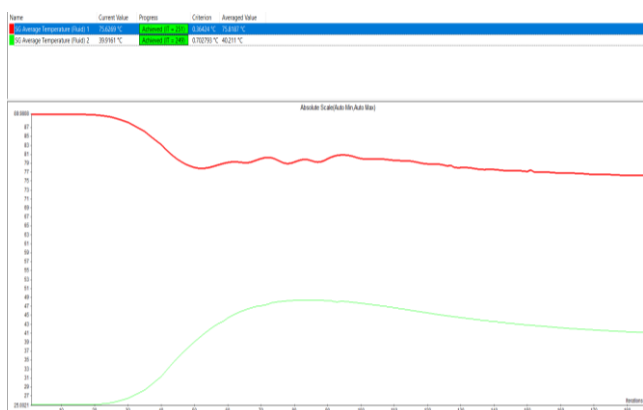
Fig -8: Temperature distribution curves for biomimetic model with sparse barbs
