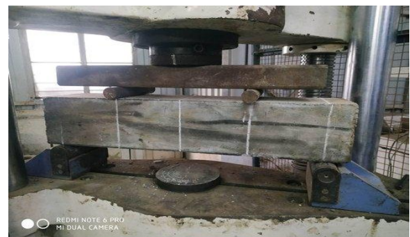
Fig-6: Flexural test of Beam
