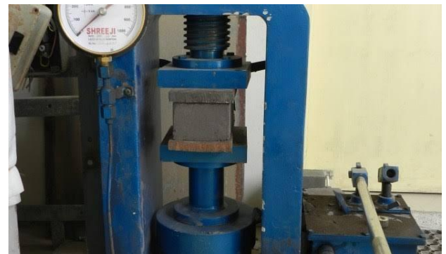
Fig-3: Compressive Test on Cube
