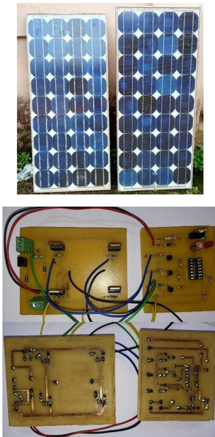
**Fig -16:** Input PV panel, Circuit connection and Etched connection
