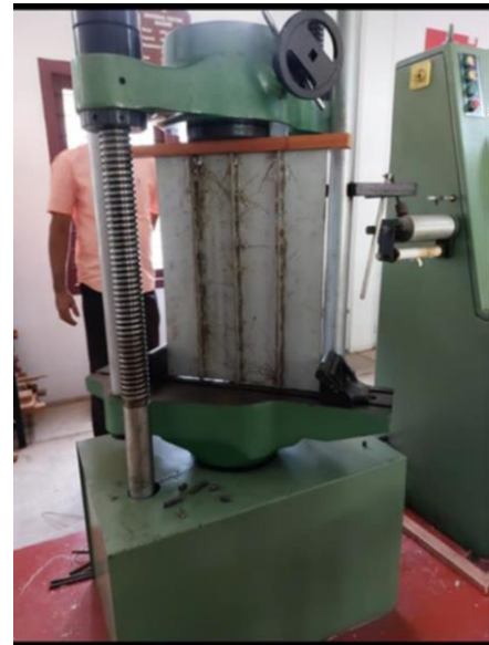
Fig -12: Applying Load on UTM
