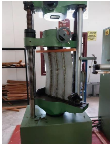
Fig -13: Deformation of stiffened plate
