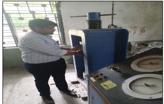
Fig 3 Laboratory compression testing machine setup
