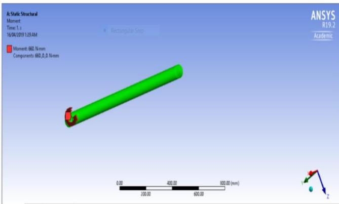
Fig. 5.5 Applying moment one end of propeller shaft
