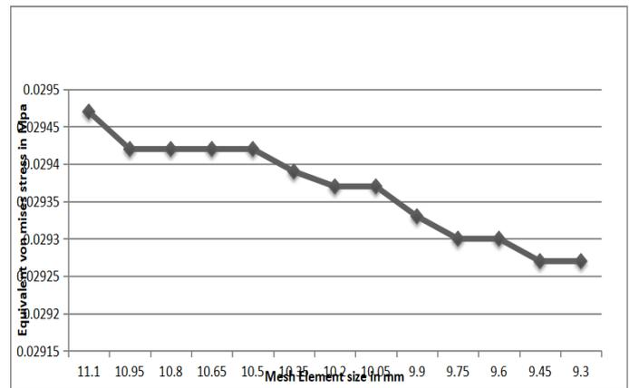
Fig -5.2 Variation in von Mises stress value with respect to the mesh size
