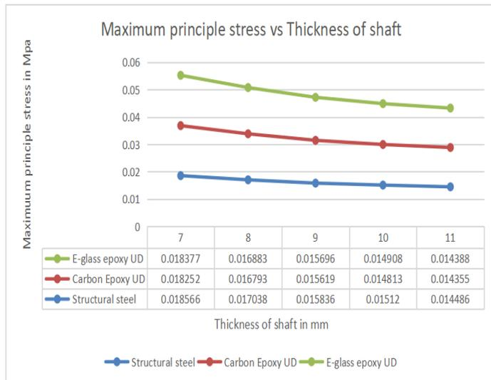
Figure 6.3 thickness vs maximum principal stress
