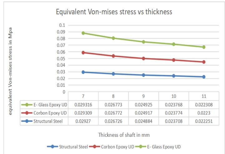
Figure- 6.1 Thickness vs equivalent (von-Mises) stress
