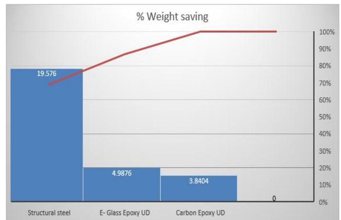
Fig.6.5 Comparison of % weigh saving of different propeller shaft
