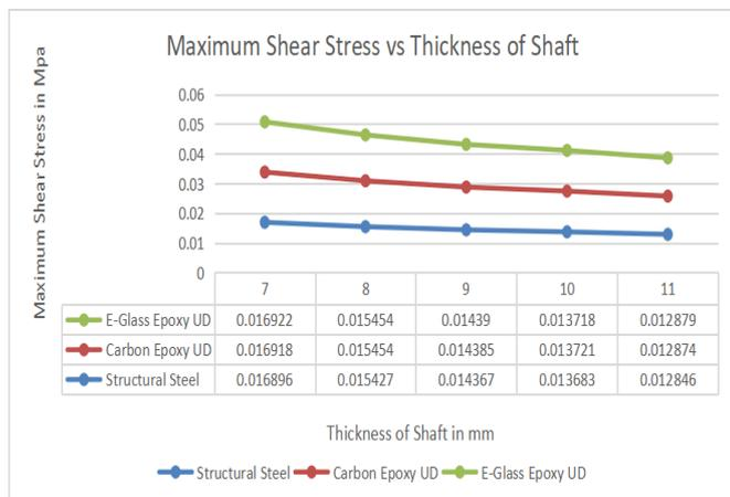
Figure 6.4 thickness vs maximum Shear stress
