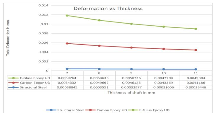
Figure 6.2 Thickness vs total displacement
