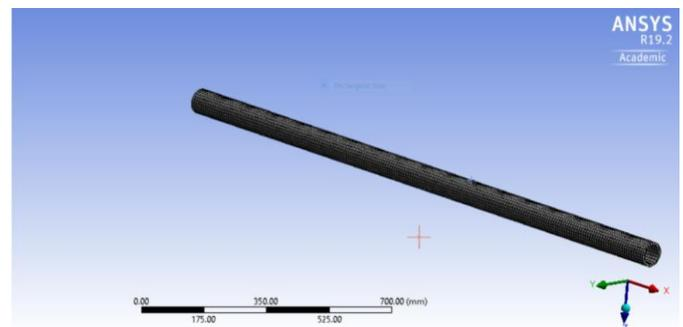
Fig.5.3 Meshed composite propeller shaft
